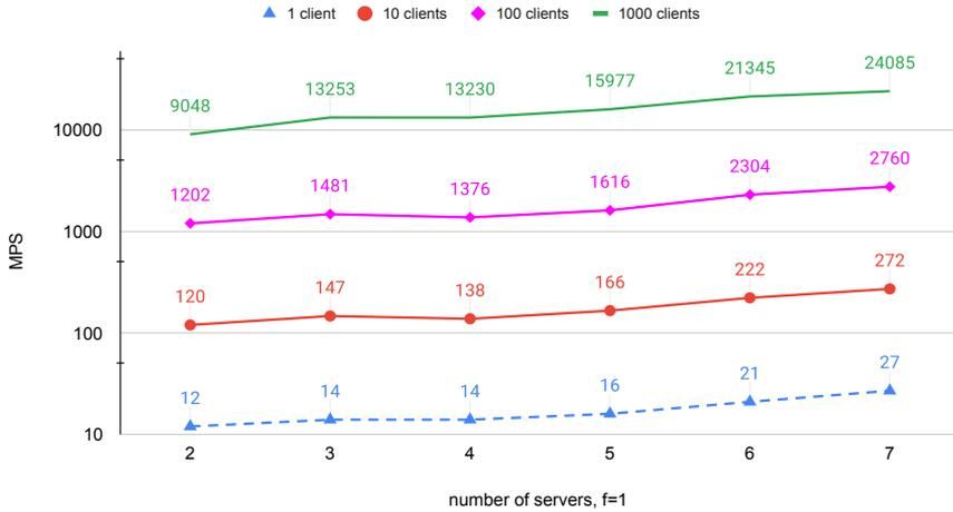
**Figure 3.4:** System throughput as a function of the number of active servers, running in different data-centers on multiple continents. Originally published in Paper D.
