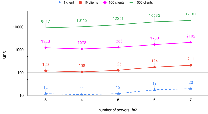
Figure 12: System throughput as a function of the number of servers, running in different data centers on multiple continents. Please note that the Y axis is logarithmic, to match the logarithmic increase in the number of clients. Here, f = 2 .
